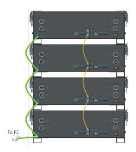
Note: the module with empty Link IN port is Master battery
