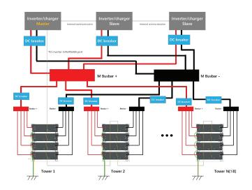
Considering system stability, when you install multiple batteries, please always keep a certain capacity margin of  $30^{\sim}50\%$ . it is recommended to configure the inverter capacity with battery energy in 1: 2 proportion, for instance, if you have a 5KW rated inverter, connect 2 pieces(10KWh) or more batteries.
